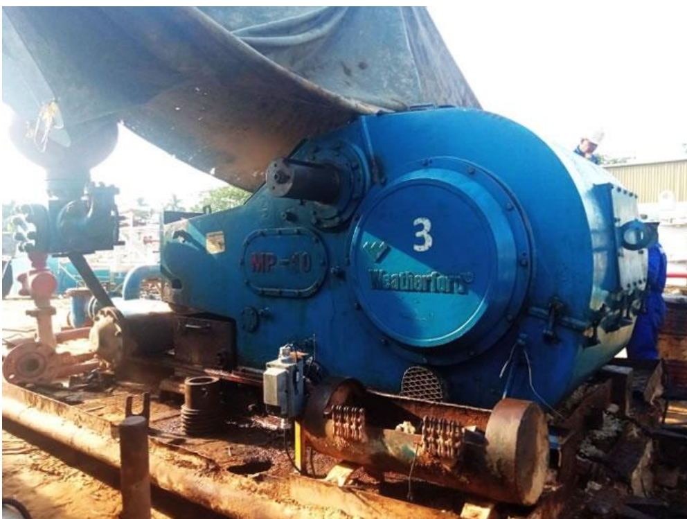
The Weatherford Mud Pump from a PT Bormindo oil drilling rig.
