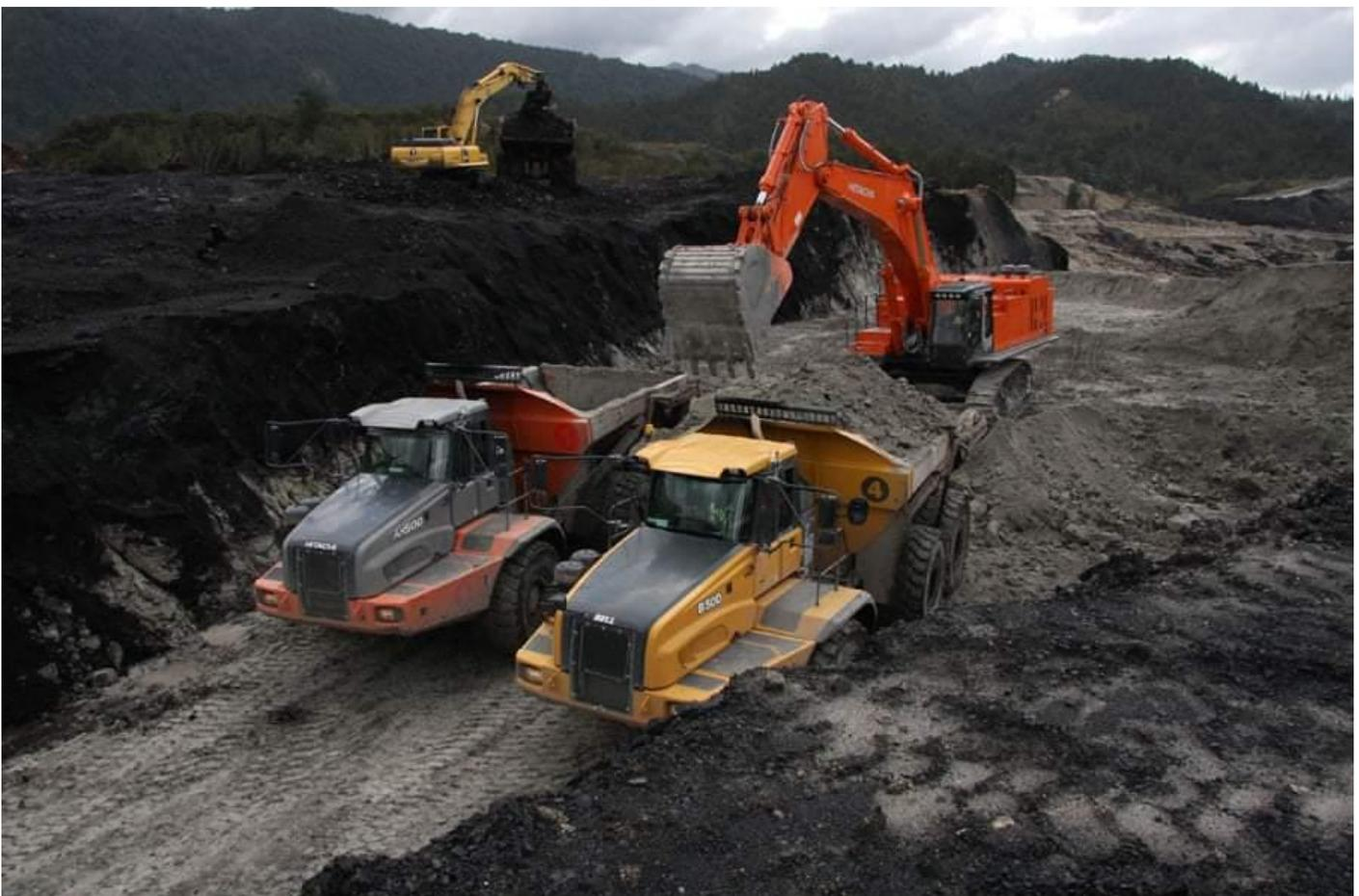
In Western Australia the operator was seeking to reduce the iron wear rate by a minimum of 10%. The use of Liquid Tungsten was trialled in one truck, a Hitachi AH500 articulated dump truck, while a similar truck, a Bell B50D, served as the control vehicle with no Liquid Tungsten added.
