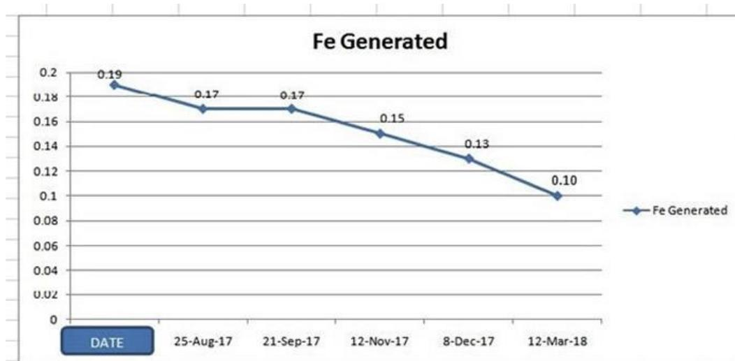
Graph of mg/l iron wear generated per oil hour
